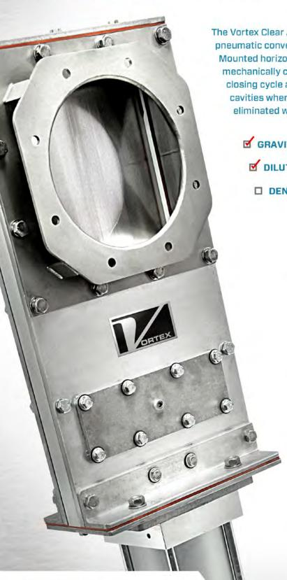
The Vortex Clear Action Gate is designed for use in gravity flow or pneumatic conveying systems up to 15 psig (1 barg) depending on size. Mounted horizontally, the machined square-edged blade of this gate mechanically clears the material from the sealing surfaces on each closing cycle allowing it to discharge beneath the valve. Open cavities where material collects in traditional gate valves have been eliminated with the square blade and seal design.
