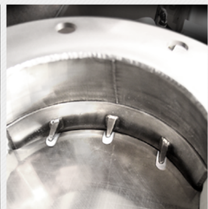
Lifting lugs and inserts provide a positive seal and prevent metal-on-metal contact
