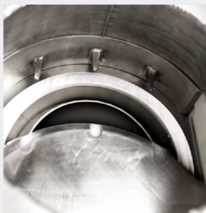
The silicone blade seal is recessed to protect it from material flow and to reduce wear
