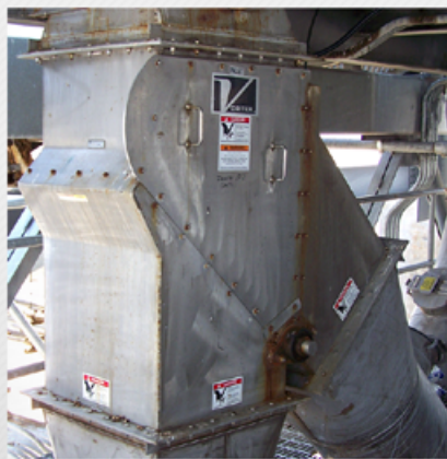
24" (610mm) straight line Seal Tite Diverter handling DDG
