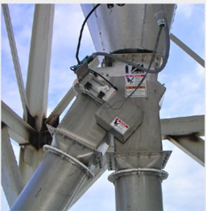
10" (254mm) straight line Seal Tite handling kaolin clay
